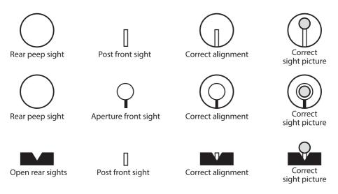
Correct sight alignment is the key to accurate shooting. Angular misalignment of the front sight with the rear sight introduces an error that is multiplied with distance.
